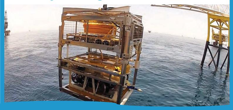
The Seaeye Cougar-XT is a compact, highly flexible and extremely powerful electric ROV with working depth of 2000 meters, proven worldwide and recognized for its capability.
